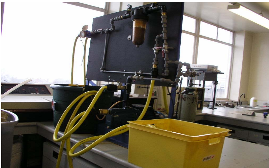
Figure 6.. Bench-scale filter to measure the attrition of the glass media under continuous operation
